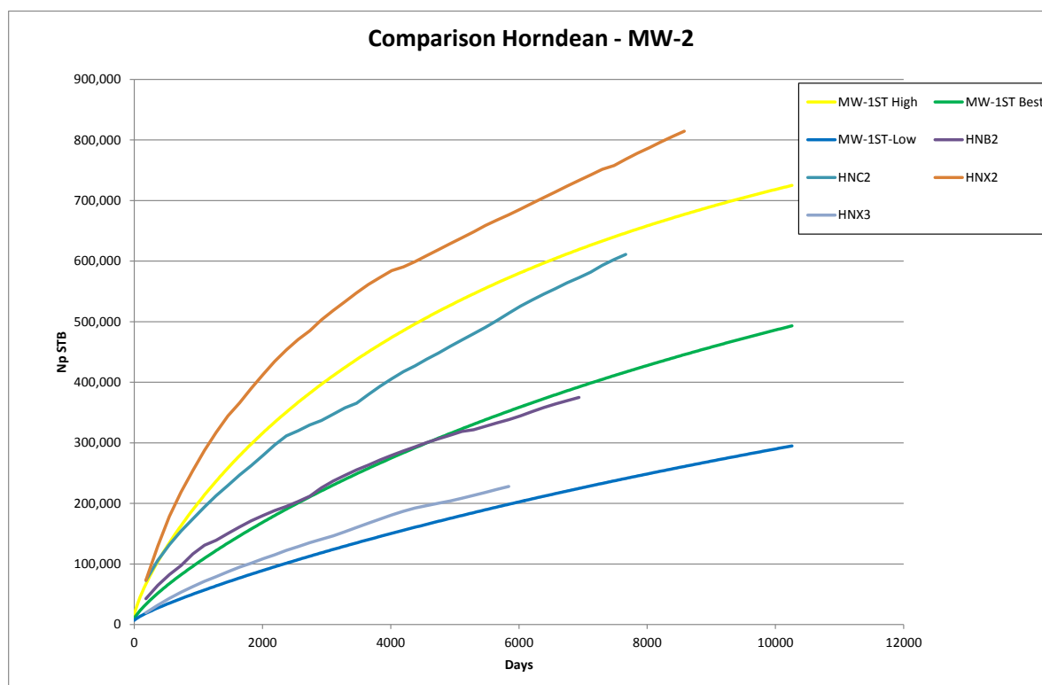
Figure 4.18 Comparison of cumulative production for the MW-1ST cases with the Horndean wells
